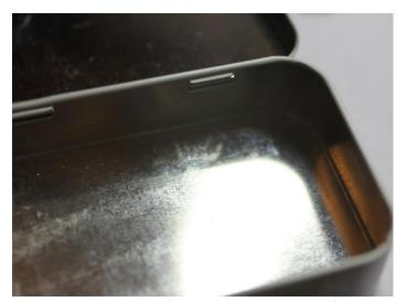
**12.** Apply a small amount of hot glue to the corner of the tin where the circuit board will be placed to hold the board still.
