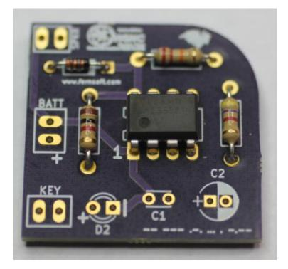
4. Insert the  $0.1 \mu F$  capacitor into C1. Solder carefully in place.
