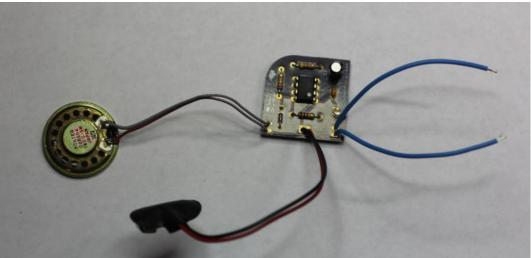
10. Insert the capacitor so that the lead marked with the white stripe (-) is in the negative position on the board, and the other lead (positive) by the plus sign on the board.
