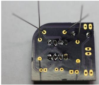
Hold the soldering iron where the resistor lead meets the through hole and solder in place using a small amount of solder. Repeat with the other leads.
