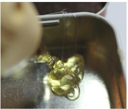
**13.** Seat the circuit board before the hot glue cools. Make sure that you use enough glue so that it prevents the board from touching the metal of the can directly. Otherwise the leads of the components with short out and your kit will not work correctly.
