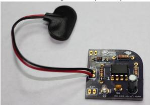
7. Connect the wire pieces provided to the pads labelled KEY as shown.
